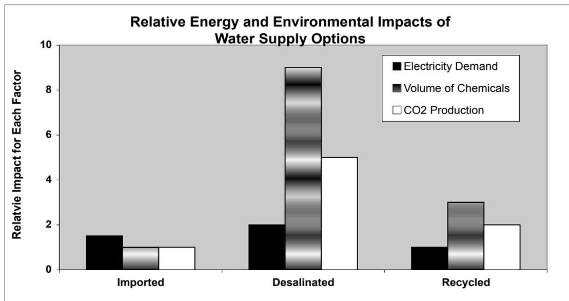
**Figure 2.** The relative energy and environmental impacts (based on the three factors of electricity demanded, volume of chemicals required, and mass of carbon dioxide produced) for various water supply options. Imported water is transported from outside the watershed, whereas desalinated and recycled water are produced from non-potable water. Based on data from Stokes and Horvath (2006) for a water purveyor in Northern California.
